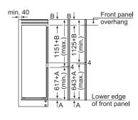
The specified unit door dimensions are valid for a door gap of 4 mm.
