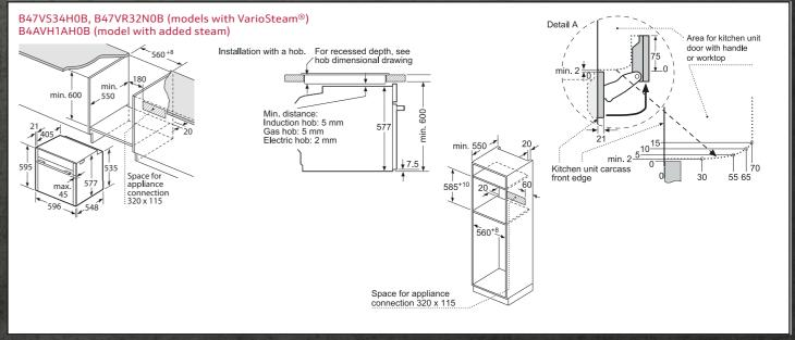
Measurements in mm. The line drawings featured in this brochure are provided as a guide to general dimensions only and are subject to amendment without prior not
