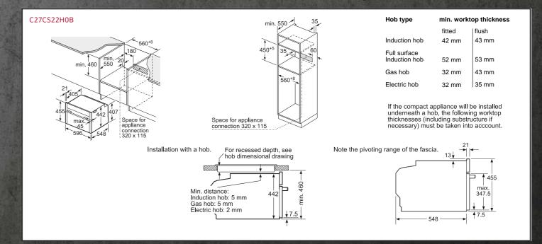
Measurements in mm. The line drawings featured in this brochure are provided as a guide to general dimensions only and are subject to amendment without prior notice For full dimensional and installation details please refer to the documentation supplied with the applianc
