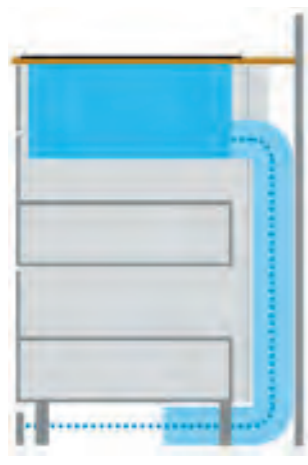
Partly ducted recirculation
