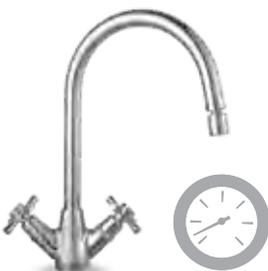
This symbol indicates the tap will work with a low pressure system, delivering at least 4 litres per minute of hot water at 0.3 bar pressure.
